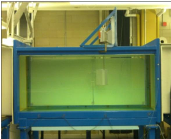
Figure 1: The RHRC 2436 water channel test section
