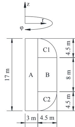
FIGURE B1. HALF OF CROSS-SECTION OF STORAGE SPACE
