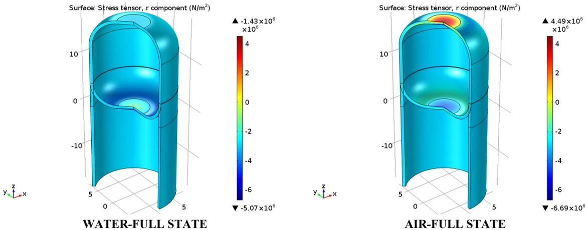
FIGURE 9. TENSILE/COMPRESSIVE STRESS IN THE CYLINDRICAL CONFIGURATON (UNIT: PA)
