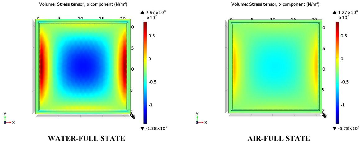
**FIGURE 7. TENSILE/COMPRESSIVE STRESS IN THE RECTAGULAR CONCRETE TANK (UNIT: PA)**
