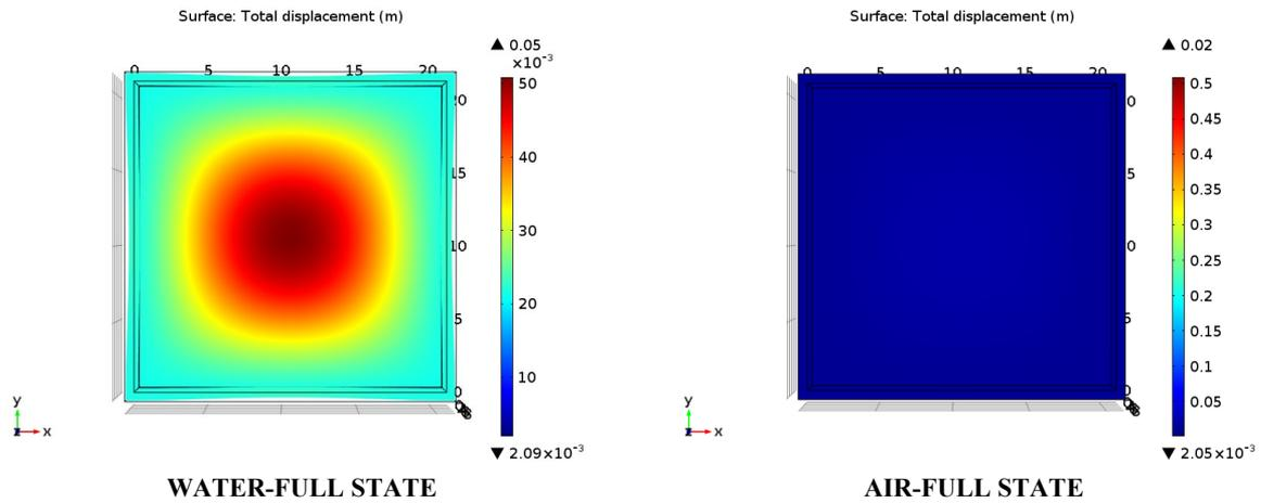
**FIGURE 6. DISPLACEMENT OF RECTANGULAR CONFIGURATION (UNIT: M)**
