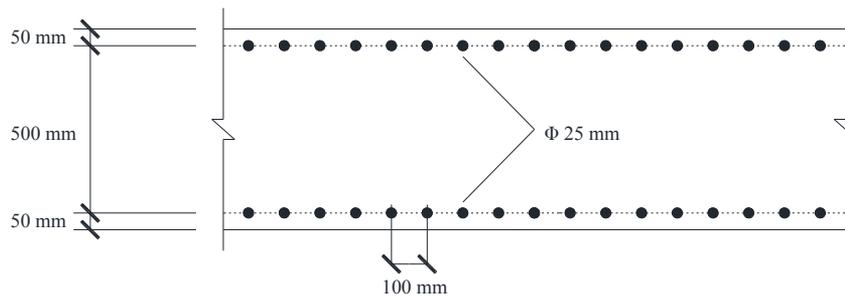
**FIGURE 3. THE REINFORCEMENT LAYOUT IN THE WALL FOR BOTH CONFIGURATIONS**
