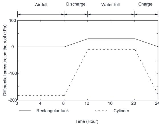
**FIGURE 5. DIFFERENTIAL PRESSURE DURING ONE OPERATIONAL CYCLE**
