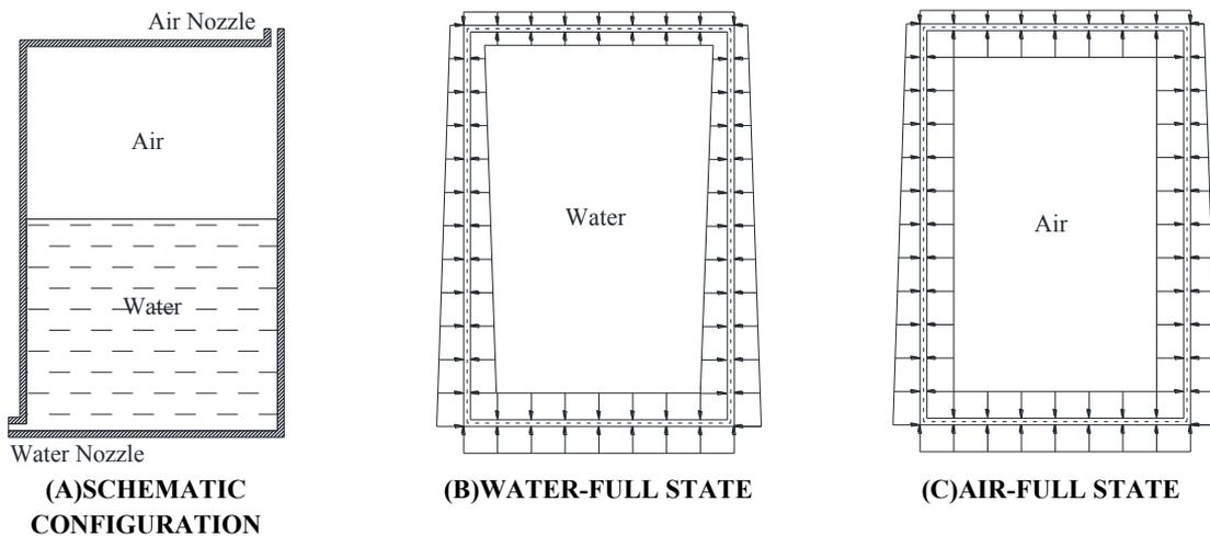
**FIGURE 4. THE SCHEMATIC CONFIGURATION OF STORAGE VESSEL AND TWO EXTREME STATES DURING ONE OPERATIONAL CYCLE**
