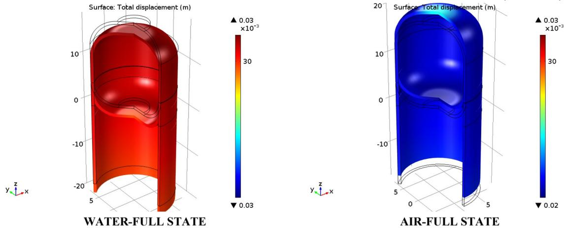
**FIGURE 8. DISPLACEMENT OF CYLINDRICAL CONFIGURATION (UNIT: M)**
