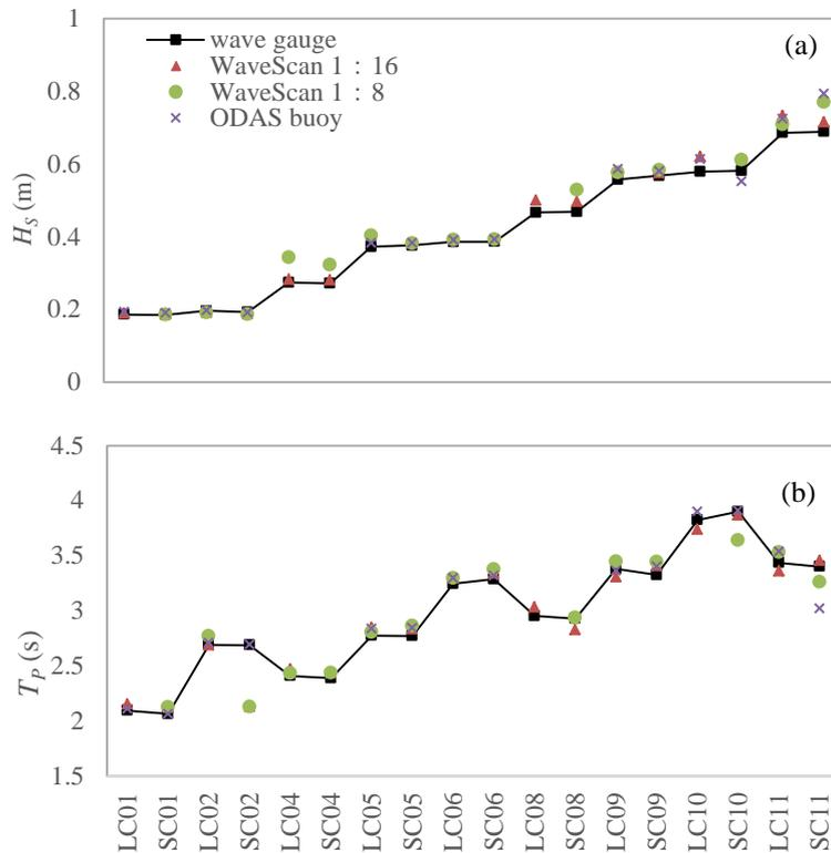
Figure 4 measurements for  $H_s$  (a) and  $T_p$  (b) during irregular wave states (LC/SC01-11)
