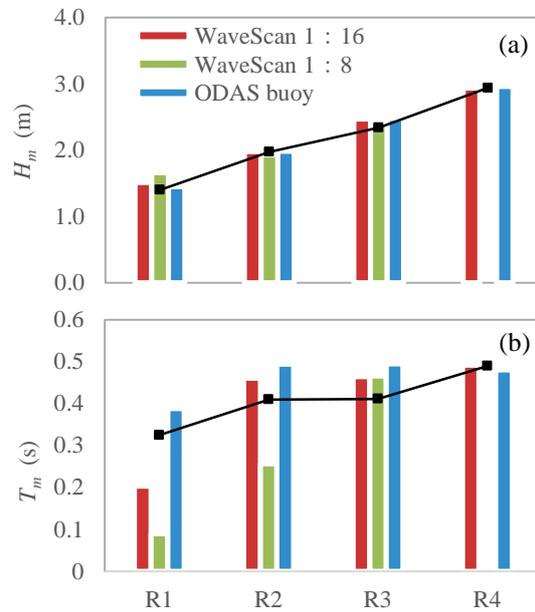
**Figure 3** measurements for  $H_m$  (a) and  $T_m$  (b) during regular wave states (R1-R4)
