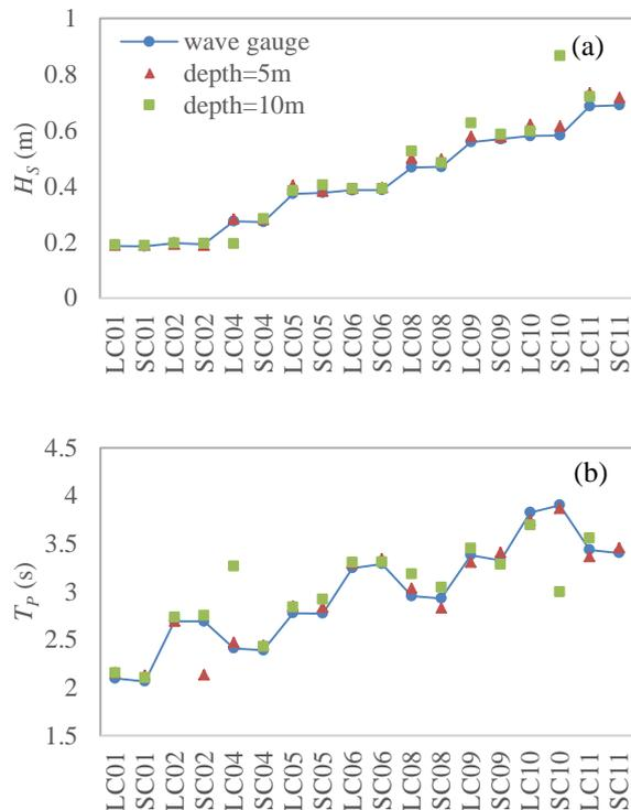
**Figure 5** Measurements for  $H_s$  (a) and  $T_p$  (b) by 1:16 Wavescan buoy model with mooring system located at depth 5m and 10m during irregular waves
