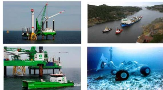
Figure 1: Top-left: Jack up platform "Neptune" ("DEME Group," 2014) installing a wind turbine at Thorntonbank OWF in 2012. Top-right: "Jules Verne" Cable Laying Vessel ("Prysmian," 2014) Bottom-left: "Aquata" Crew Transfer Vessel ("DEME Group," 2014) at Thorntonbank OWF in 2012. Bottom-right: "Hydro Plow" submarine trencher ("Prysmian," 2014)
