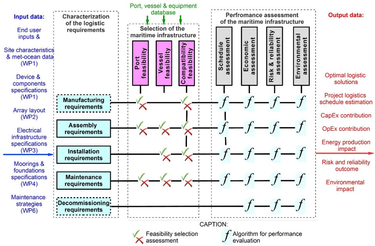
Figure 4: Flow-chart of the lifecycle logistics model in DTOcean
